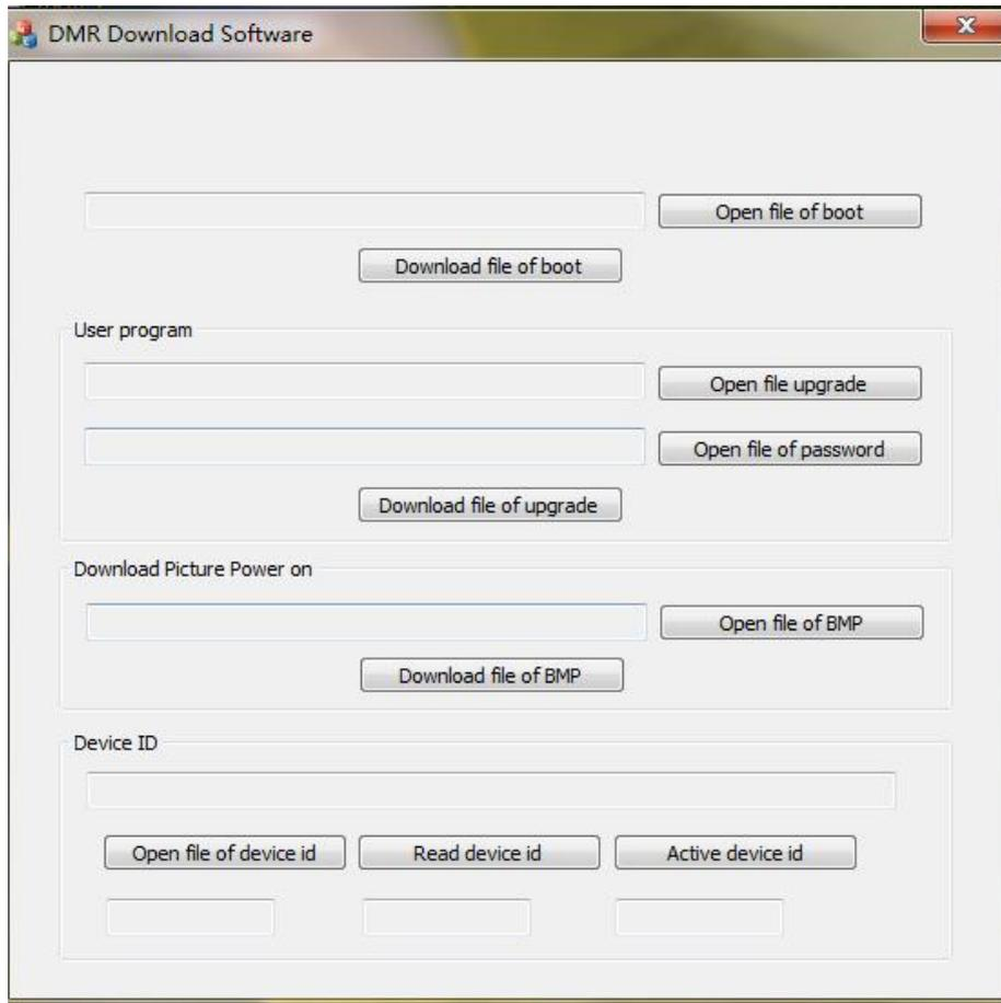
And then write upgraded file into radio, the radio will be upgraded as following:
